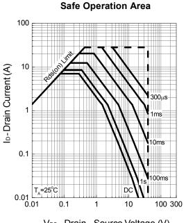
V<sub>DS</sub> - Drain - Source Voltage (V)
