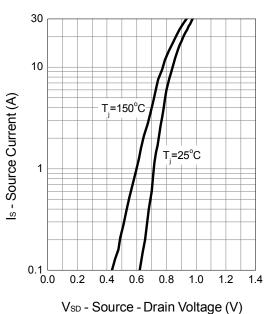
Source-Drain Diode Forward
