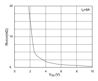
Fig.2 On-Resistance vs. Gate-Source
