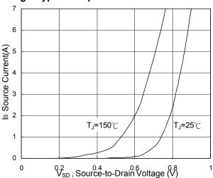
Fig.3 Forward Characteristics Of Reverse
