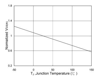
Fig.5 Normalized  $V_{GS(th)}$  vs.  $T_J$
