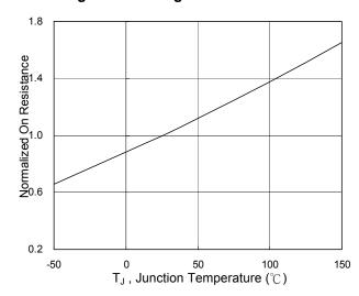
Fig.6 Normalized R<sub>DSON</sub> vs. T<sub>J</sub>
