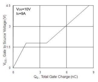
Fig.4 Gate-Charge Characteristics
