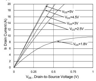
**Fig.1 Typical Output Characteristics**
