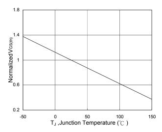
Fig.5 Normalized  $V_{\text{GS(th)}}$  vs.  $T_{\text{J}}$
