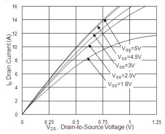
**Fig.1 Typical Output Characteristics**
