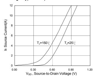
Fig.3 Forward Characteristics Of Reverse
