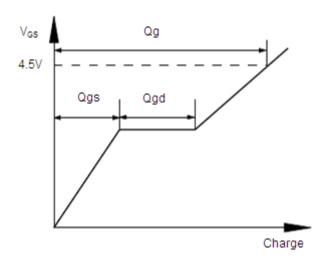
Fig.11 Gate Charge Waveform
