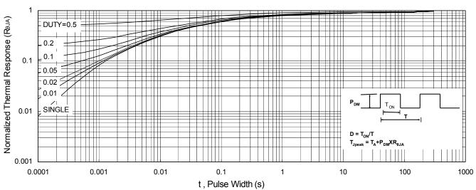
Fig.9 Normalized Maximum Transient Thermal Impedance
