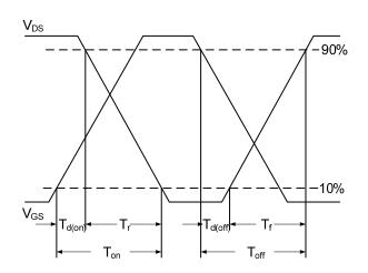
Fig.10 Switching Time Waveform
