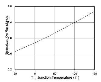
Fig.6 Normalized R<sub>DSON</sub> vs. T<sub>J</sub>
