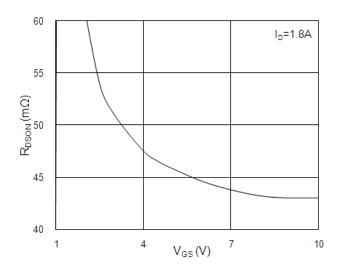
Fig.2 On-Resistance vs. Gate-Source
