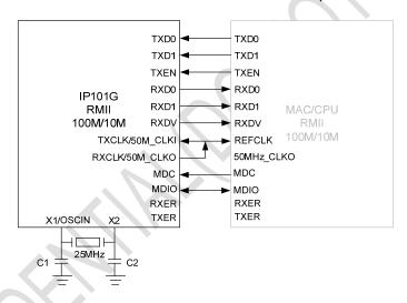
Figure 8 IP101G RMII Mode with internal clock Block Diagram
