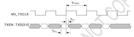
Figure 19 MII Transmit Timing Requirements
