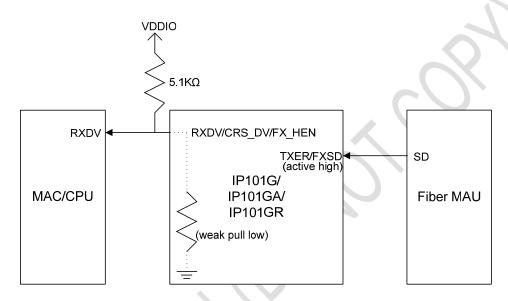
Figure 17 IP101G Fiber Mode Setting
