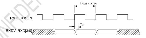
Figure 22 RMII Receive Timing Specifications
