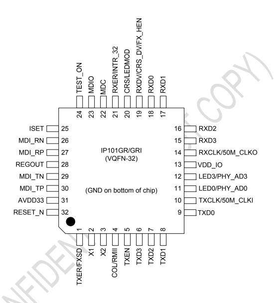
Figure 3 IP101GR/GRI 32 Pin Diagram
