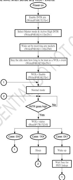
Figure 14 Sleep or wake up automatically programming guide
