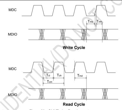
Figure 23 SMI Timing Requirements
