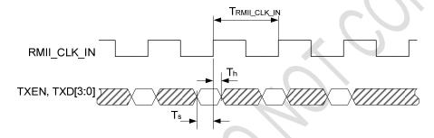
Figure 21 RMII Transmit Timing Requirements
