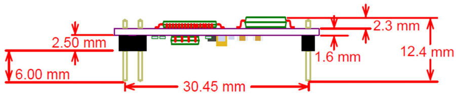
Figure 1-2 W5500S2E-S1 dimension - side view
