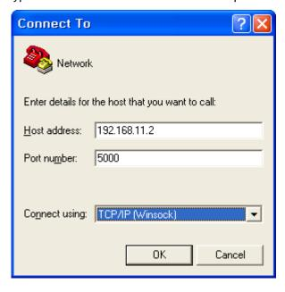
Figure 18. Network Terminal Program configuration
