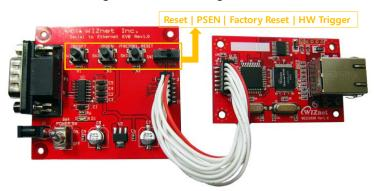
Figure 2. WIZ105SR Configuration Environment Setting Diagram
