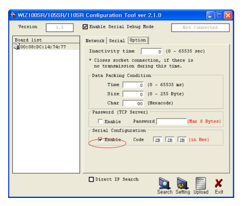
Figure 14. Serial Configuration Enable Setting
