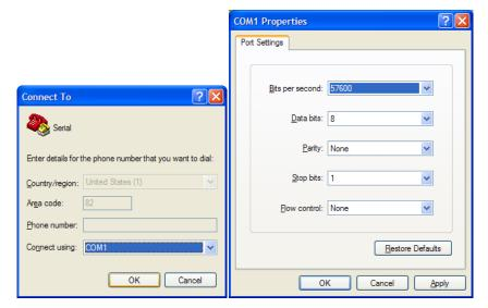
Figure 17. Serial Terminal Program configuration
