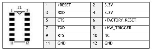
Figure 1. WIZ105SR Connector Pin Assignment and Definition
