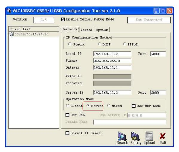
Figure 9. Operation Mode for Password Setting
