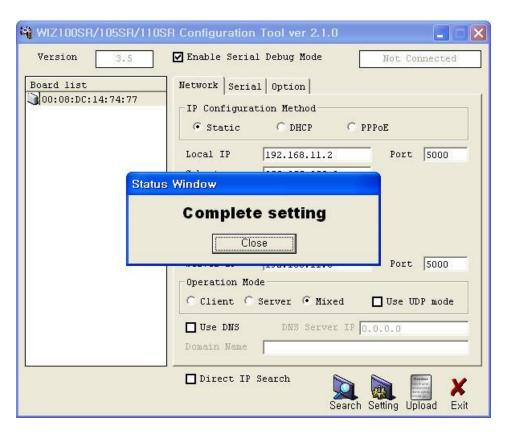
Figure 16. Result Window after Running "Setting"
