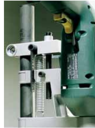
depth of cut set by depth stop
