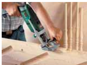
tiltable double guide bars with scale for drilling +/- 45°
