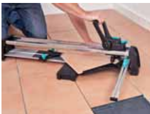
special guide for diagonal cutting
