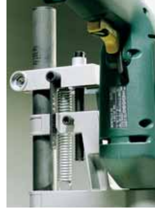
depth of cut set by depth stop
