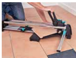
special guide for diagonal cutting
