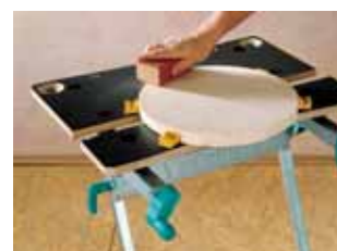
plastic jaws for securing the workpiece horizontally
