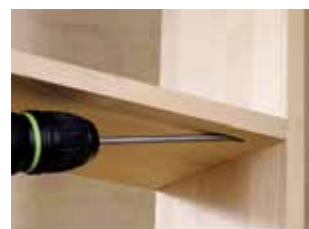
...then you join the two workpieces with wood screws...
