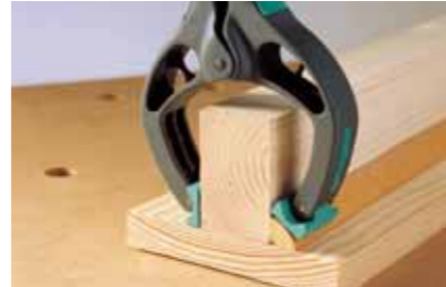
movable clamping jaws adjust to the workpiece
