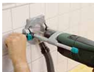
grab handle for precise placement and against skidding when drilling
