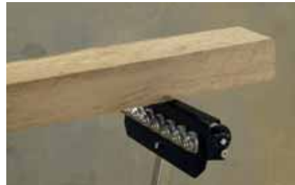
the stable support is used for extending the bearing surface of a work table and for supporting long work pieces
