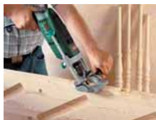
tiltable double guide bars with scale for drilling +/- 45°
