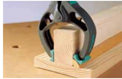
movable clamping jaws adjust to the workpiece
