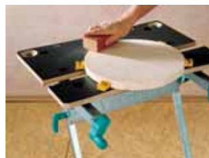
plastic jaws for securing the workpiece horizontally
