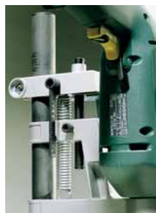
depth of cut set by depth stop
