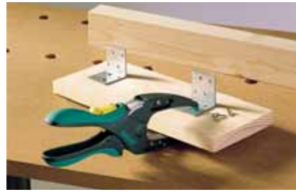
large depth offered by the long clamp arms allows fixing in areas far away from the edge of the workpiece
