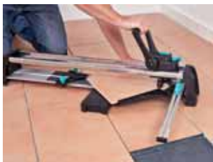
special guide for diagonal cutting
