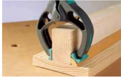
movable clamping jaws adjust to the workpiece
