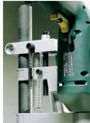
depth of cut set by depth stop
