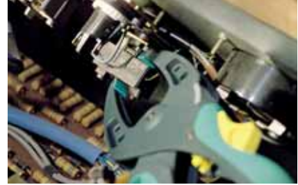
long tapered clamp arms will make fixing in confined spaces easy
