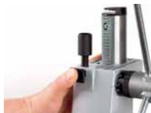
depth adjustment by means of a depth stop with quick adjuster
