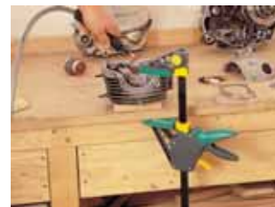
effortless conversion to the spreading function
