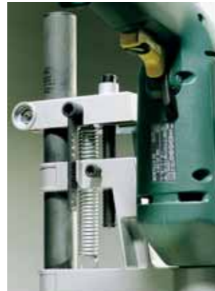
depth of cut set by depth stop
