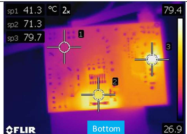
Figure 16. Thermal image of bottom layer at 850VDC input and full load
