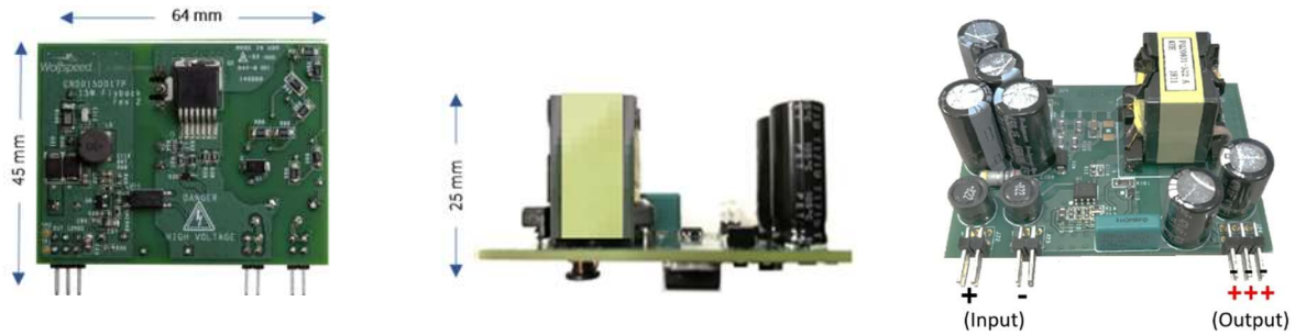
Figure 2. Physical Dimensions and Pinouts of Cree's CRD15DD17P, 15 W flyback auxiliary power supply board
