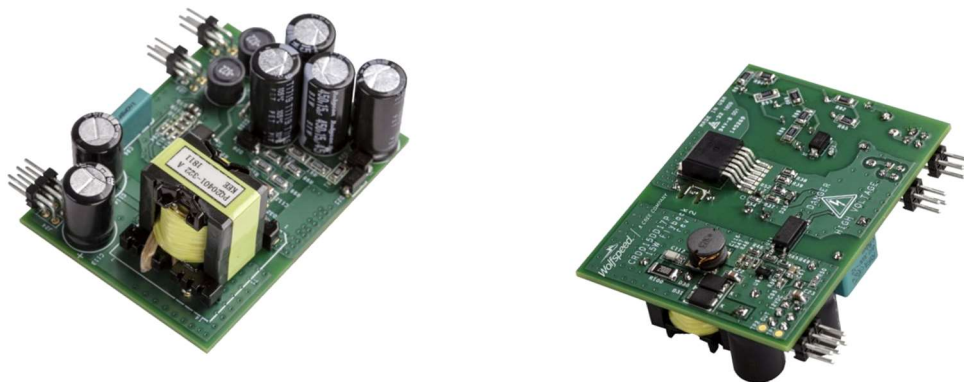
Figure 1. Cree's CRD15DD17P, 15 W flyback auxiliary power supply board
