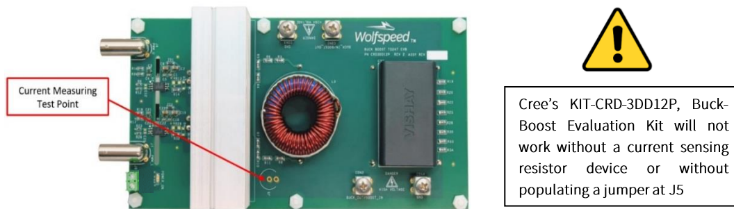
Figure 17. Current Measuring Test Point on Cree’s KIT-CRD-3DD065P/CRD-3DD12P Buck-Boost Evaluation Kit
