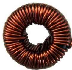
Figure 8. Inductor of Cree’s KITCRD-3DD12P Buck-Boost, Evaluation Kit
