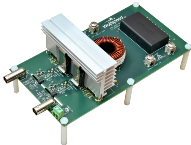
Figure 1. Cree's KIT-CRD-3DD065P/CRD-3DD12P, Buck-Boost Evaluation Kit
