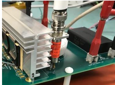
Figure 16. Cree’s KIT-CRD-3DD065P/CRD-3DD12P, Buck-Boost Evaluation Kit with Current Viewing Resistor Installed
