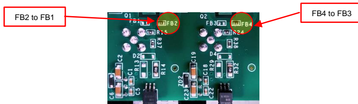
Figure 15. Location of Resistors on the top side of PCB
