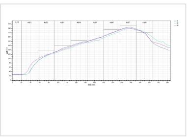
Remarks: 1. All temperatures referred are measured on the surface of the package body.
