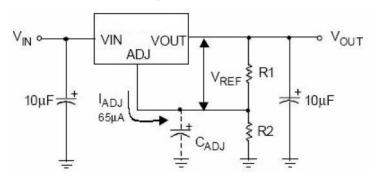
Figure 1. Basic Adjustable Regulator
