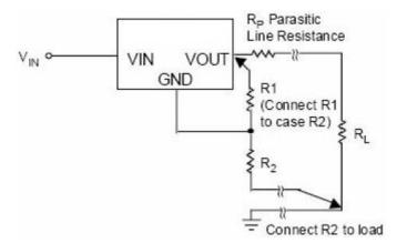
Figure 2. Best Load Regulation Using Adjustable Output Regulator
