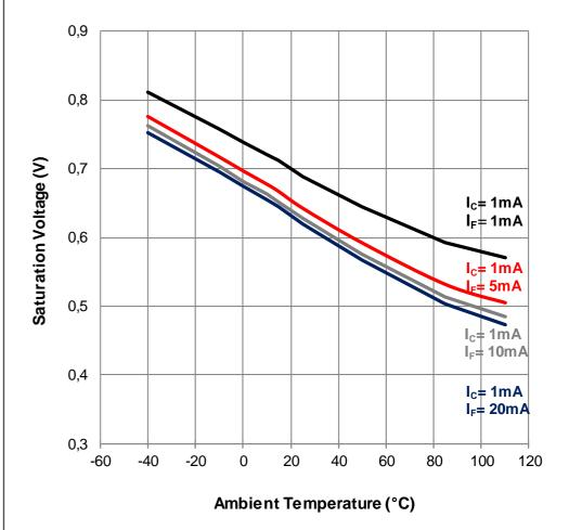
Testcondition:  $I_F = 1$  mA; normalized to  $T_{\Delta} = 25$  °C
