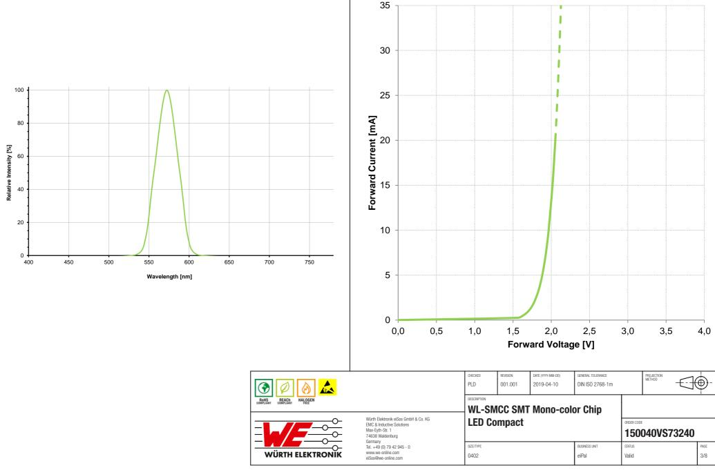
Forward Current vs. Forward Voltage:
