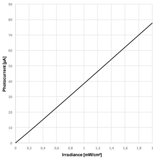
Testcondition: Ee=0,5mW/cm<sup>2</sup>, VR=5V
