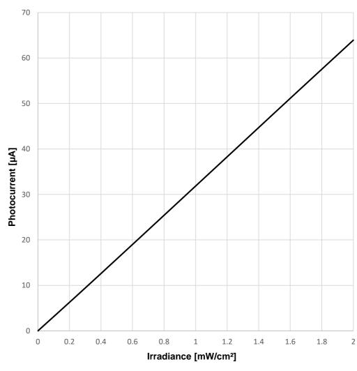
Testcondition: Ee=0,5 mW/cm<sup>2</sup>; VR=5V
