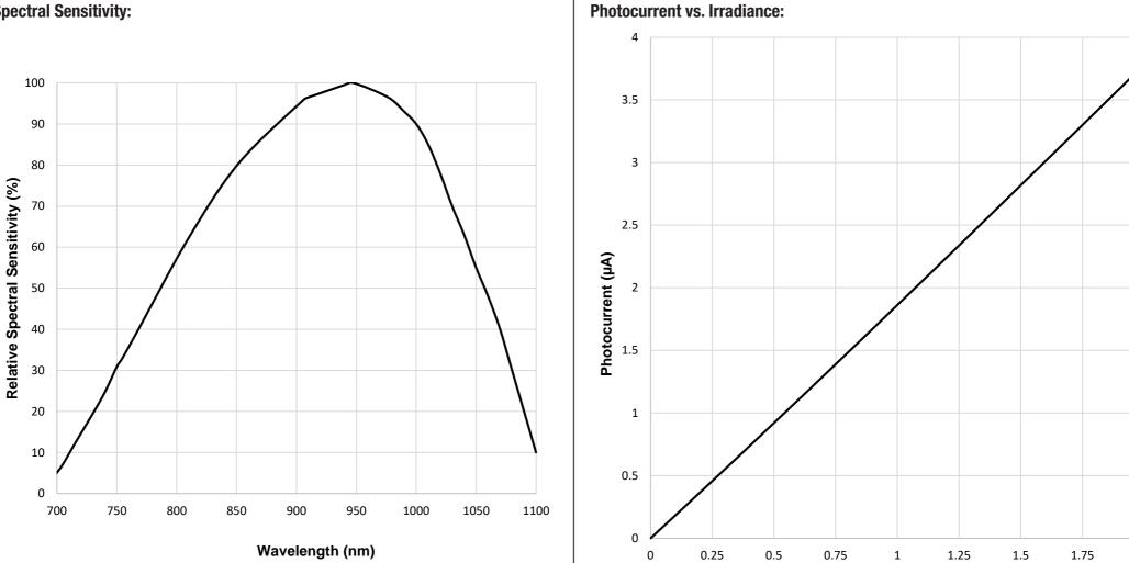
Testconditon: Ee=0,5mW/cm<sup>2</sup>; VR=5V
