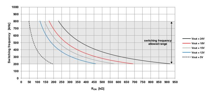
As stated above, the off-time is also limited to a minimum value of 260 ns, which limits the maximum duty cycle. Larger  $R_{ON}$  (lower  $F_{SW}$ ) should be selected in any application requiring large duty ratio.
