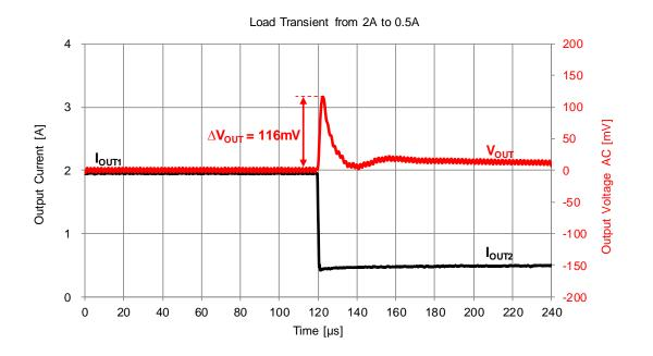
In both the positive and the negative transition, the  $\Delta V_{OUT}$  is below the target (120mV).
