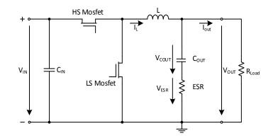
None of the required output capacitors are integrated within the module. A general recommendation in order to guarantee a stable behavior is to place at least a capacitance of  $10\mu$ F (MLCC recommended) at the output. The output capacitor must meet the worst case RMS current rating, as calculated by equation (8):
