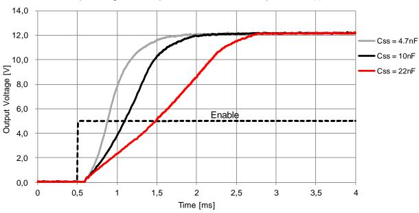
Output Voltage at Start Up with Different Soft-Start Capacitors at V<sub>OUT</sub> = 12V
