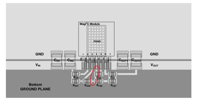
The ground connections for the soft-start capacitor (Css), the output voltage lower resistor divider (R<sub>FBB</sub>) and enable components (when used) should be routed to the AGND pin of the device. If not properly handled, poor grounding can result in degraded load regulation or erratic output voltage ripple behavior. Place C<sub>SS</sub>, R<sub>FBT</sub> and R<sub>FBB</sub> close to their respective pins.
