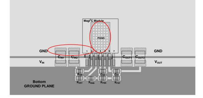
The negative terminal of  $C_{IN1}$  and  $C_{IN2}$  needs to be very close to the PGND pad of the power module.
