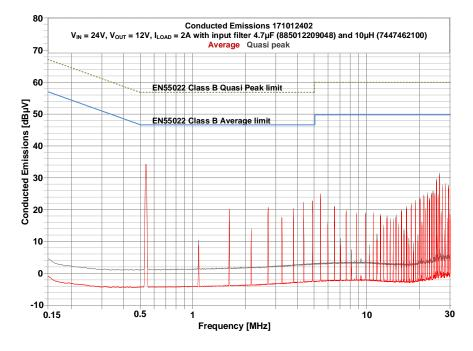
Magl<sup>3</sup>C Power Module VDRM – Variable Step Down Regulator Module
