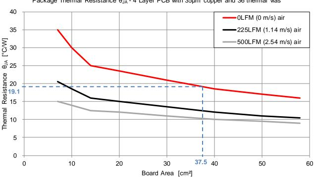
Package Thermal Resistance  $\theta_{JA}$  - 4 Layer PCB with 35µm copper and 36 thermal vias
