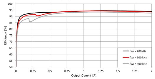
Efficiency vs Frequency,  $V_{IN} = 24V$ ,  $V_{OUT} = 12V$ ,  $T_A = 25^{\circ}C$
