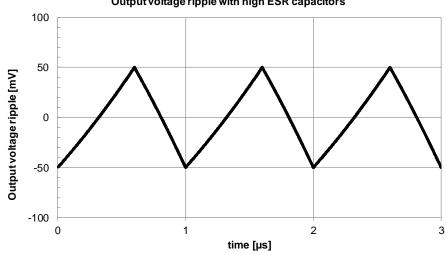
Output voltage ripple with high ESR capacitors
