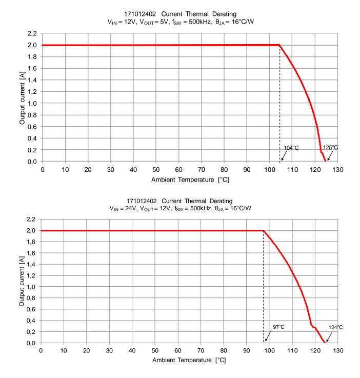
The ambient temperature and the power limits of the derating curve represent the operation at the max junction temperature specified in the "Operating Conditions" section on page 4.
