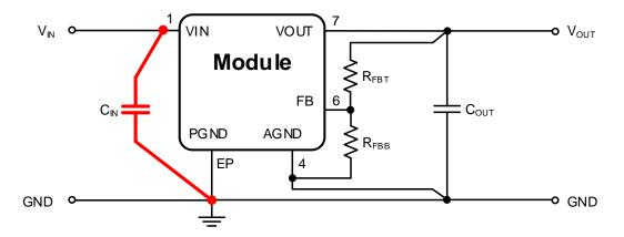
Based on those considerations, the path of the input capacitor  $C_{IN}$  is the most critical one to generate high frequency noise on  $V_{IN}$ . Therefore place  $C_{IN}$  as close as possible to the Magl<sup>3</sup>C power module  $V_{IN}$  and PGND exposed pad EP. This will minimize the high di/dt area and reduce radiated EMI. Additionally, grounding for both the input and output capacitor should consist of a localized top side plane that connects to the PGND exposed pad.
