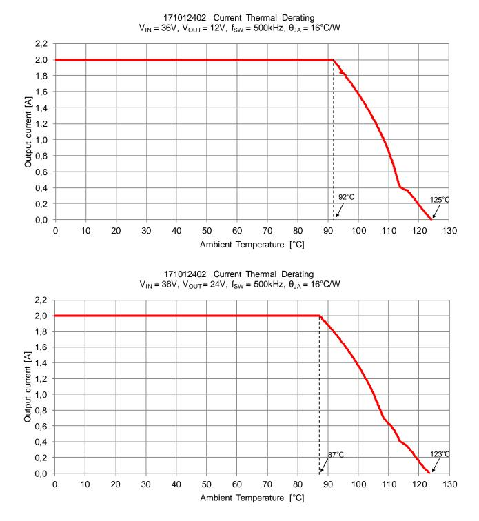
The ambient temperature and the power limits of the derating curve represent the operation at the max junction temperature specified in the "Operating Conditions" section on page 4.
