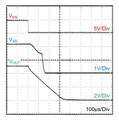
Figure 9. EN shutdown Iout = 2A
