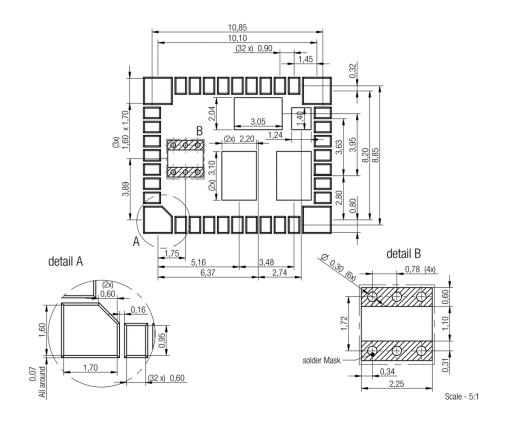
recommended soldering pad solder past recommendation 150  $\mu m$
