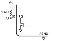
$V_{CC} = V_{IN}$  or other supply voltage below 5.5V
