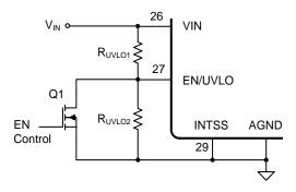
Figure 7. Typical Enable/Disable Control
