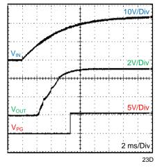
Figure 3. Startup  $V_{IN}$ =10V;  $I_{OUT}$ =2A
