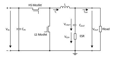
None of the required output capacitors is integrated within the module. At a minimum, the output capacitor must meet the worst case RMS current rating of  $0.5 * \Delta I_L$ , as calculated in equation (4).
