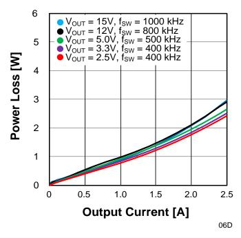
From the graph we read a power loss of 1.5W. Adding 20% results in a loss of 1.8W. Entering the values in formula (16) results in:
