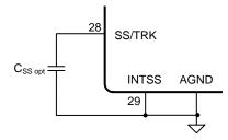
Figure 4. Soft-Start Capacitor Css and INTSS connection
