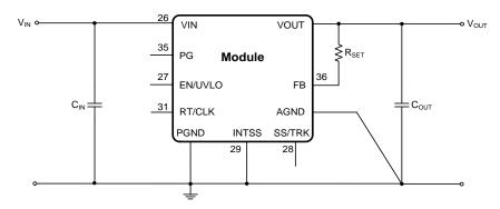
Figure 2. Basic Soft-Start configuration
