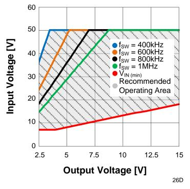
Figure 1. Input Voltage vs. Output Voltage Operating Area
