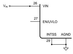
Figure 5. EN/UVLO configuration without resistive divider
