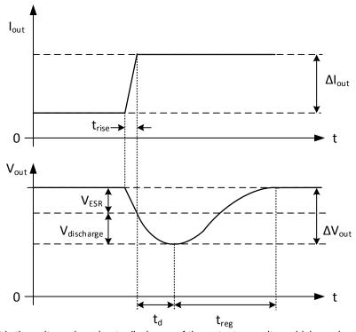
The second component is the voltage drop due to discharge of the output capacitor, which can be estimated as:
