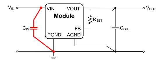
Based on those considerations, the path of the input capacitor  $C_{IN}$  is the most critical one to generate high frequency noise on Vin. Therefore place  $C_{IN}$  as close as possible to the Magl<sup>3</sup>C power module  $V_{IN}$  and PGND pins. This will minimize the high di/dt area and reduce radiated EMI. Additionally, grounding for both the input and output capacitor should consist of a localized top side plane that connects to the PGND pins.
