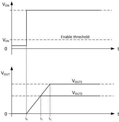
Figure 11. Simultaneous voltage tracking waveforms
