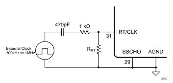
Figure 12. Synchronization Configuration
