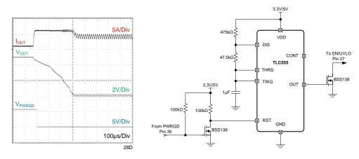
Figure 14. Overcurrent Limiting
