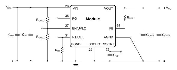
Recommended component values specified at  $T_A = 25$ °C
