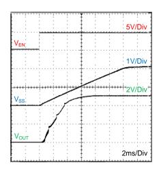
Figure 8. EN start-up I<sub>OUT</sub> = 2A
