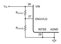
Figure 6. Undervoltage Lockout (UVLO) Schematic
