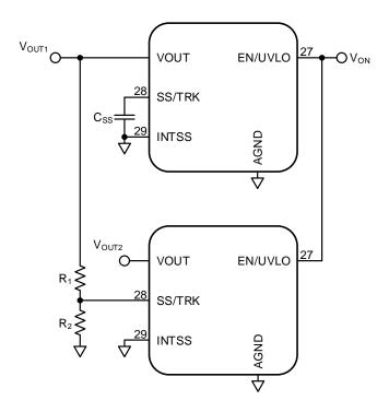
Figure 10. Voltage tracking configuration
