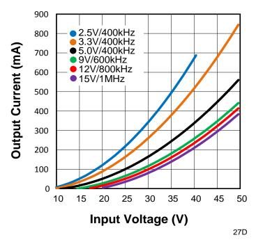
Figure 13. Pulse Skipping Load Threshold
