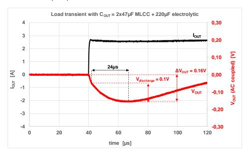
In order to have a safer margin from the desired  $\Delta V_{OUT}$ <0.1V, additional capacitance at output would be required.
