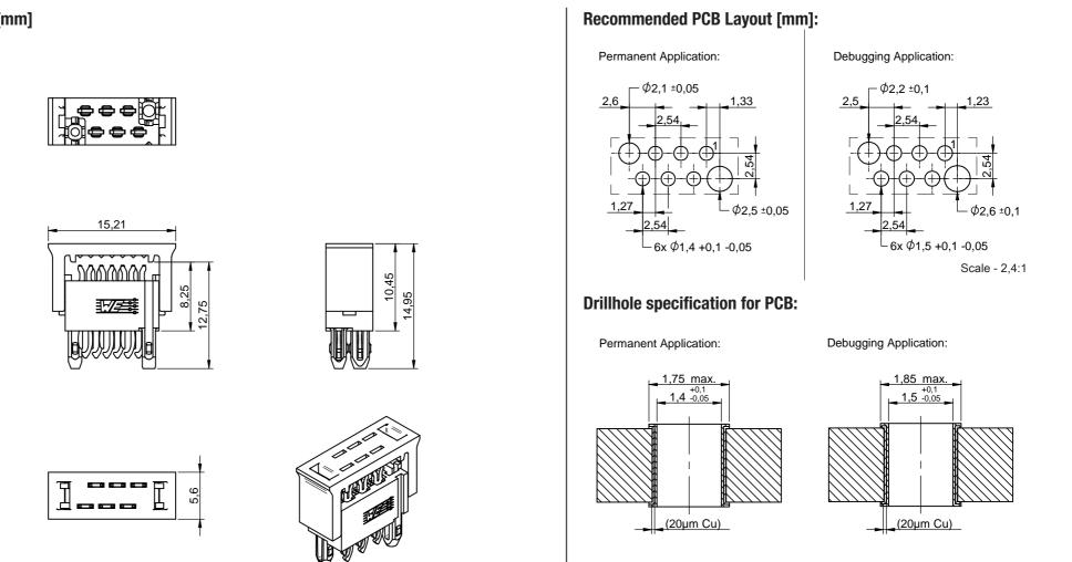
Drill hole specification for chemical surfaces (Ni/Au)
