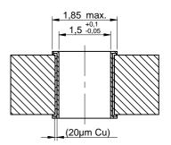
Drill hole specification for chemical surfaces (Ni/Au)
