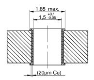
Drill hole specification for chemical surfaces (Ni/Au)
