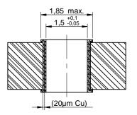
Drill hole specification for chemical surfaces (Ni/Au)
