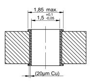
Drill hole specification for chemical surfaces (Ni/Au)
