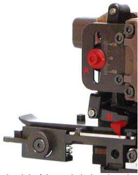
For adapting the pawl B to the pitch of the terminals, in order to have a new terminal correctly placed on the anvil for each cycle of the press: loosen the nut A and move the screw up for a greater pitch or down for a shorter one. Then tighten the nut again.
