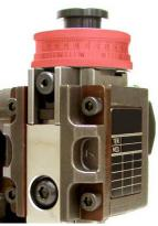
Free the brake by means of the lever B, place the terminals in the guide A, push it until it will be hooked by the pawl C and then tighten the brake by means of the lever B.
