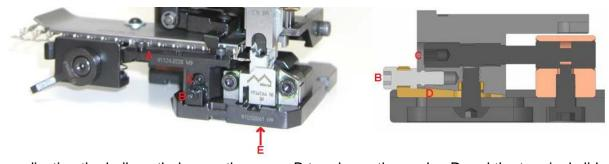
For adjusting the bellmouth, loosen the screw B to release the wedge D and the terminal slide A. Rotate screw C clockwise or counter-clockwise to obtain the desired adjustment. Tighten B again until D blocks A.
