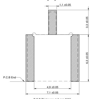
P.C.B Thickness: 1,6 mm MAX Scale - 8:1
