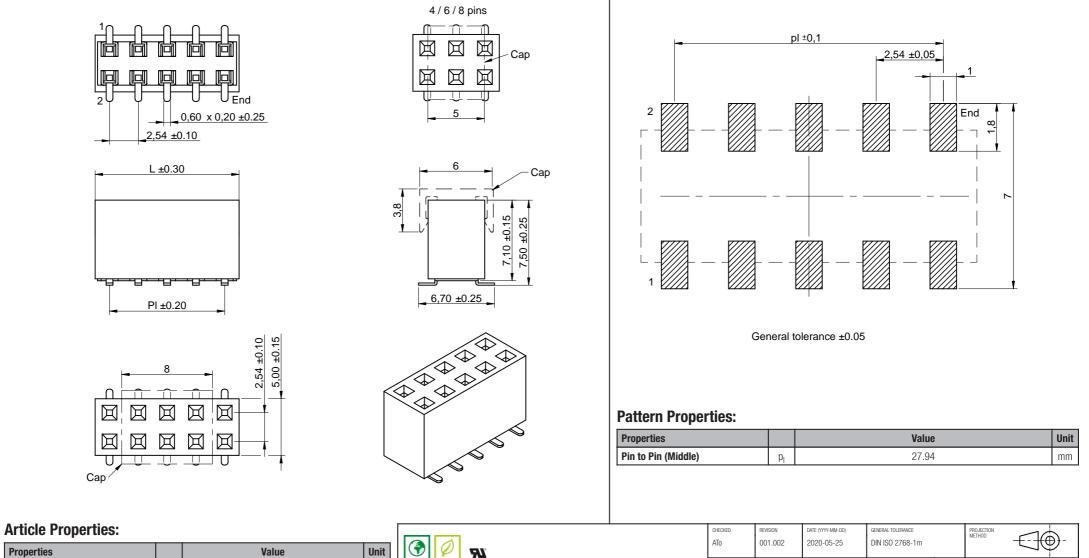
Properties Pins 24 Pin to Pin (Middle) 27.94 P Length 30.98 L
