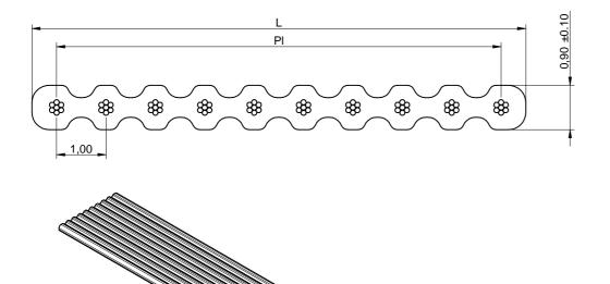
Note: Because of manufacturing matters, our Ribbon flat cable reels might be cut into two pieces. Please note that Würth Elektronik won't accept any complaint or replacement about that.
