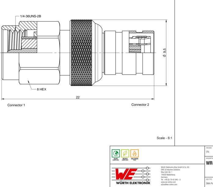
PROJECTION METHOD REVISION DATE (YYYY-MM-DD) GENERAL TOLERANCE €₩ 001.000 2020-04-30 DIN ISO 2768-1m DESCRIPTION **WR-ADPT Coax Adaptor** ORDER CODE 64403216211000 SIZE/TYPE BUSINESS UNIT STATUS PAGE 1/6 SMA Plug to SMB Plug eiCan Valid
