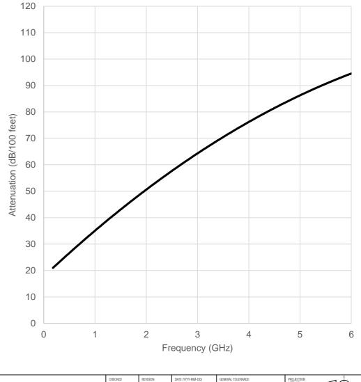
JaC 001.000 2019-03-13 DIN ISO 2768-1m **WR-CXASY SMA Bulkhead Jack to** Würth Elektronik eiSos GmbH & Co. KG **MMCX Straight Plug** EMC & Inductive Solutions Max-Eyth-Str. 1 74638 Waldenburg 65503260515305 Germany Tel. +49 (0) 79 42 945 - 0 BUSINESS UNIT www.we-online.com **WÜRTH ELEKTRONIK** 3/5 Valid Flexible Cable RG-316/U eiCan eiSos@we-online.com
