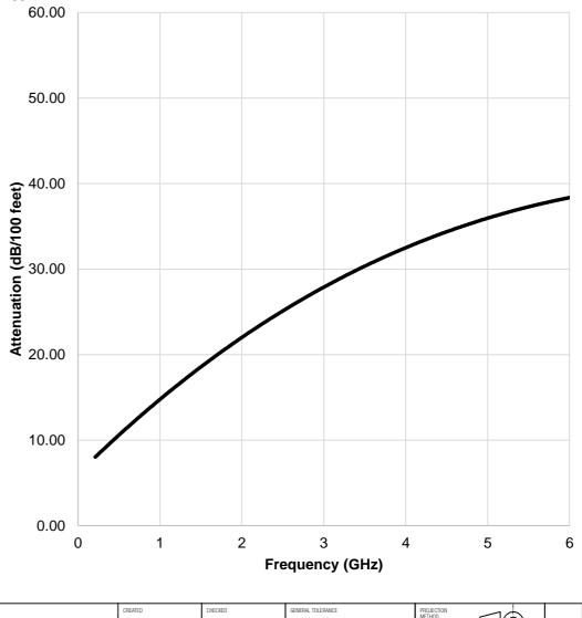
Würth Elektronik eiSos GmbH & Co. KG <del>-(1)</del> DaSc EMC & Inductive Solutions JTs DIN ISO 2768-1m Max-Eyth-Str. 1 74638 Waldenburg SMA Straight Plug to SMA Right Tel. +49 (0) 79 42 945 - 0 Angle Plug on Flexible Cable RG142 www.we-online.com 65503503630502 **WR-CXASY** eiSos@we-online.com STATUS 001.000 Valid 2018-03-19 eiCan 3/5
