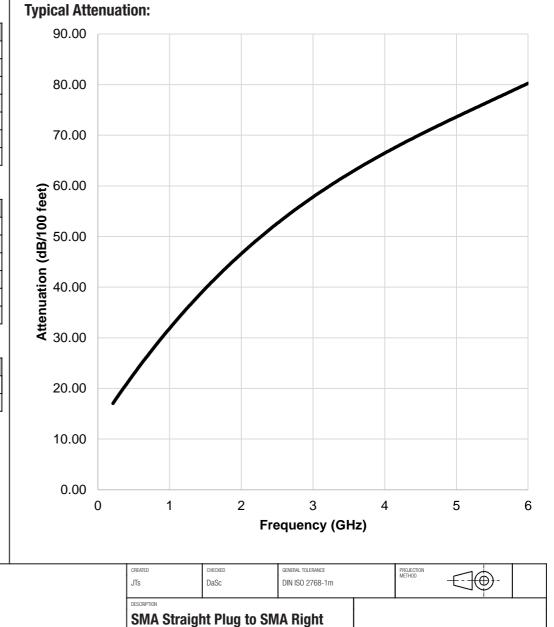
Angle Plug on Flexible Cable RG316
