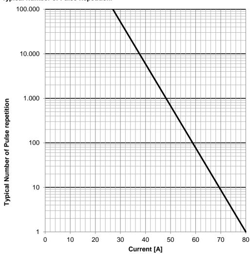
valid for ambient temperature: +25°C; 8 ms pulse length, single pulse valid for ambient temperature: +25°C; 8 ms pulse length, 10 s break between pulse
