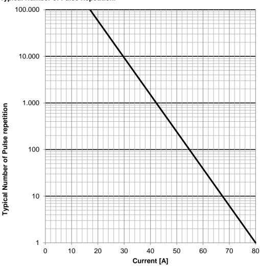
valid for ambient temperature: +25°C; 8 ms pulse length, single pulse
