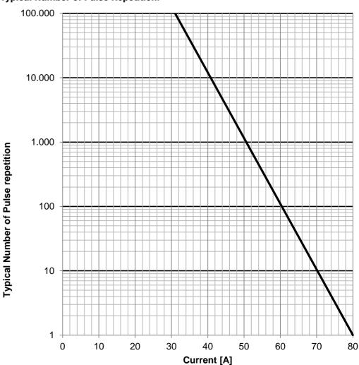
valid for ambient temperature:  $+25^{\circ}\text{C}$ ; 8 ms pulse length, single pulse
