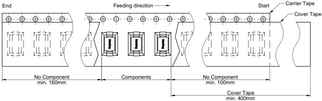
W2 detail B Cover Tape Chip Cavity Sprocket Hole
