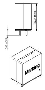
Pin 2 and 3 are only for mechanical stability.
