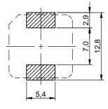
no sensitive traces underneath the component
