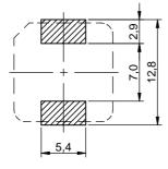
no sensitive traces underneath the component
