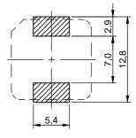
no sensitive traces underneath the component
