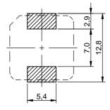
no sensitive traces underneath the component
