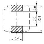
no sensitive traces underneath the component
